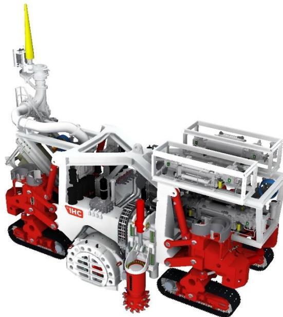
*Arctic Canadian Diamond Company and IHC Mining’s Underwater Mining Crawler for the Underwater Remote Mining System. The crawler will help recover diamond-bearing kimberlite ore from deep open pits at the Ekati Diamond Mine, in the Northwest Territories of Canada.*
